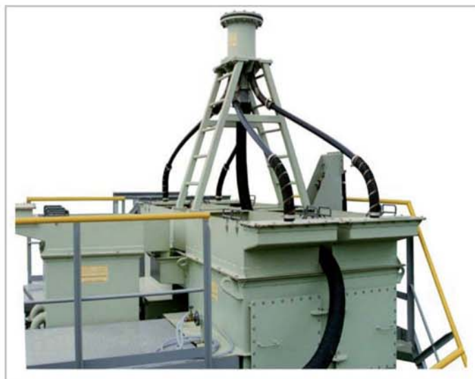
BSP-10 Alluvial Bulk Sample Plant Winner of an Australian BHP Steel Award for excellence in design and innovation, Primary Industry Category, Incorporating the Model J3 Russell Jig
